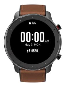
To exit the battery saver mode, long press any button on the watch.
