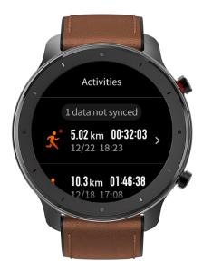
To delete a workout record on the watch, tap to enter the workout record details page, slide up to the bottom of the page, and then tap the delete button.
