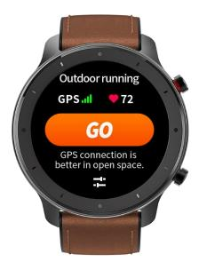
If it takes a long time to process positioning, it may be because the buildings nearby block satellite signals, or because the watch is disconnected to the App for a long time, causing the AGPS to be not upgraded. You can open the Amazfit App, connect it to the watch, and try again after the AGPS is updated.
