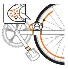
Spin the wheel counterclockwise to pass the Speed Sensor Sensing Point. The Test Key LED should start flashing if the device is installed properly.
