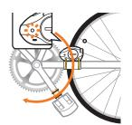
Turn the crankarm clockwise to pass the Cadence Sensor Sensing Point. The Test Key LED should start flashing if the device is installed properly.
