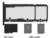
Replace the SIM/SD card slot and push down until it clicks into place.
